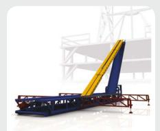
Step 3: Tubular carriage to drill floor position
