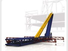
Step 4A: Fixed-carriage handles tubulars to drill floor - heights up to 24 feet
