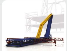
Step 4B: Hinged-carriage handles tubulars to drill floor - heights up to 32 feet
